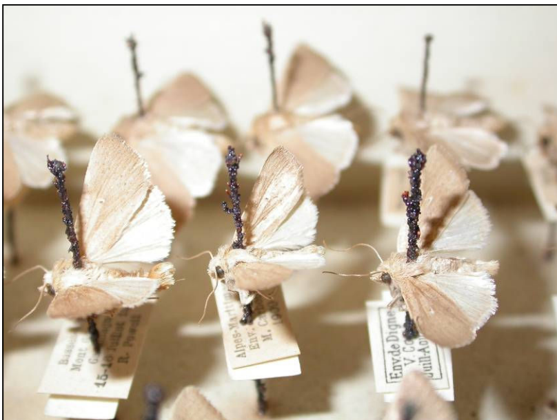
Fig. 3. Rust formation on non-stainless steel pins.
