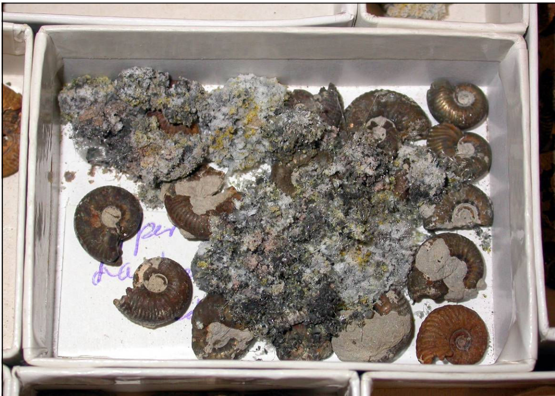
Fig. 1. A card tray (approximately 140 mm long) of small fossilised Jurassic ammonites, preserved partly in pyrite. Many have suffered from pyrite oxidation, as evidenced by the mass of grey and yellow powder covering most of the specimens.
