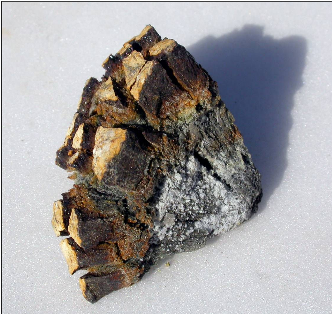
Fig. 4. A fragment (approximately 60 mm across) of a nodule of radiating pyrite after significant pyrite decay. There are two symptoms of pyrite decay in evidence: the white crystalline powder on the internal face to the right of the image, and the deep cracks in the external surface of the specimen, on the left of the image, where sections of the external surface have pulled away from one another as the specimen has expanded.
